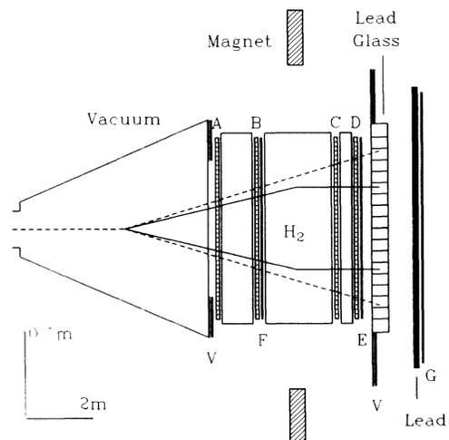
FIG. 1. Schematic plan view of the E845 detector. The neutral beam enters from the left. Note the different horizontal and vertical scales.
