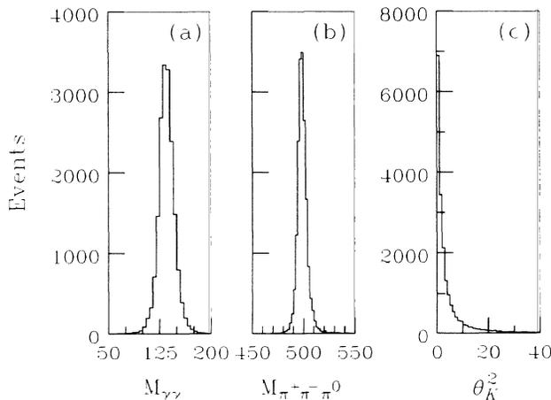
FIG. 2. For a sample of  $K_L \rightarrow \pi^+ \pi^- \pi^0$  decays the distributions of (a) the  $\gamma\gamma$  effective mass ( $\text{MeV}/c^2$ ); (b) the  $\pi^+ \pi^- \pi^0$  effective mass ( $\text{MeV}/c^2$ ); and (c)  $\theta_K^2$ , the square of the target reconstruction angle ( $\text{mrad}^2$ ).
