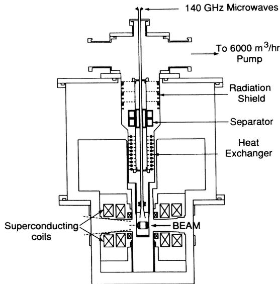
FIG. 1. Diagram of the new polarized-proton-target apparatus. The superconducting magnet produces a highly uniform 5-T field. The  $^4\text{He}$  cryostat produces about 0.9 W of cooling power at 1 K. The target material is contained in the small cavity at the bottom of the cryostat. The 140-GHz microwaves are fed into the target cavity via the horn. The proton beam will pass through the target cavity.
