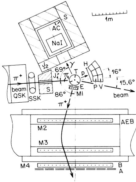
FIG. 1. Experimental setup. AEB, pion spectrometer magnet; QSK, quadrupole triplet; SSK, horizontal steering magnet; S, shielding;  $J_1, J_2$ , beam-monitor telescope (above beam plane);  $M1-M4$ , multiwire proportional chambers; T, polarized target; A, B, E, trigger-counter banks in pion spectrometer; H, P, V, proton hodoscope, total absorption, and veto counters; NaI, 64-fold photon-detector matrix; AC, cosmic-ray and charged-particle veto counters.
