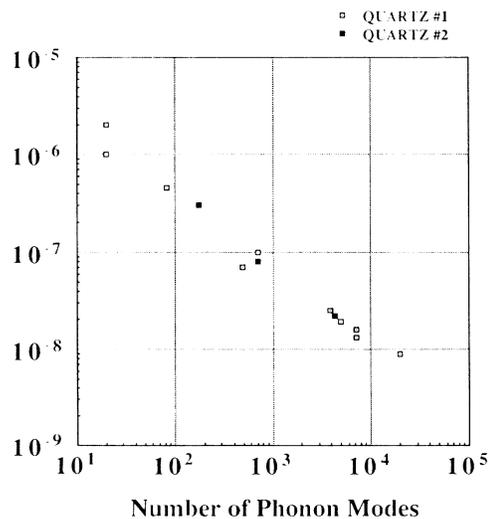
FIG. 3. Dependence of the  $1/f$  spectrum at 1 Hz on the number of phonon modes involved in the scattering.
