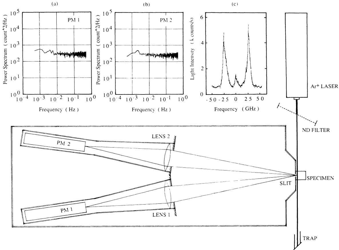
FIG. 1. Experimental setup. Insets (a),(b): PSD of dark counts of photomultipliers 1 and 2. Inset (c): An optical PSD of scattered light.
