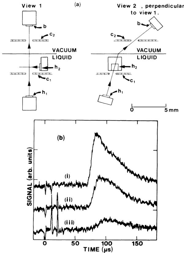
FIG. 2. (a) The experiment shown schematically from two viewpoints perpendicular to each other. The probe roton pulse is generated by  $h_1$ , and the scattering pulse by  $h_2$ . At the liquid surface the probe rotors evaporate atoms which travel to bolometer  $b$ . (b) Typical signal shapes received; the probe-pulse power is constant at  $2 \text{ mW mm}^{-2}$ . The scattering-heater power is 0, 1.26, and  $5.00 \text{ mW mm}^{-2}$  in (i), (ii), and (iii), respectively.
