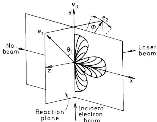
FIG. 1. Schematic diagram of the experimental geometry. The  $3p_x$  and  $3p_y$  charge-cloud distributions are indicated. The polar angles are  $\theta_1 = \theta_2 = 45^\circ$ . The out-of-plane azimuthal angle  $\phi$  of detector 2 is varied to vary the momentum  $k_x$ .
