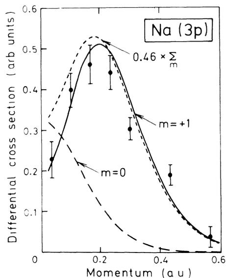
FIG. 4. The measured and calculated momentum profiles for the excited  $3p$  state of Na. The solid curve is the calculated  $3p(m_l=+1)$  profile, the short-dashed curve the total  $3p(m_l=0 \pm 1)$  profile, and the long-dashed curve that expected for the  $m_l=0$  component. The PWIA calculations use a Hartree-Fock  $3p$  wave function (Ref. 13) with the experimental angular resolution folded in. The momentum is probed along the  $k_x$  axis, with  $\bar{k}_y = \bar{k}_z = 0$ .
