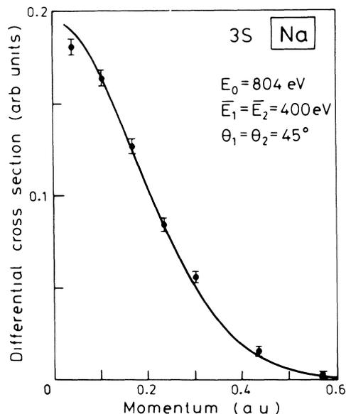
FIG. 3. The 800-eV noncoplanar symmetric momentum profile for the  $3s^{-1}$  orbital of sodium, compared with the Hartree-Fock wave function of Clementi and Roetti (Ref. 12). The finite experimental angular resolution has been folded into the calculated momentum profile. The mean summed emitted electron energy is 800 eV, the incident energy being 804 eV.
