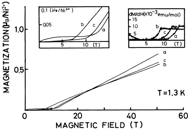
FIG. 1. The magnetization curves along the crystalline  $a$ ,  $b$ , and  $c$  axes of NENP obtained at  $T=1.3$  K. Inset (left): Low-field part of the magnetization curves. Inset (right): Corresponding  $dM/dH$  vs  $H$  curves obtained in the pulsed-field experiment. If we take the midpoints of the steplike  $dM/dH$  curves, the values of the transition fields along the  $a$ ,  $b$ , and  $c$  axes are 13, 7.5, and 11 T, respectively.
