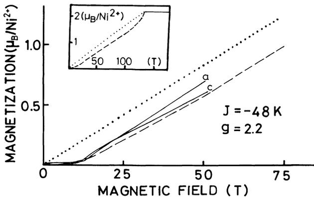
FIG. 2. The magnetization curves of NENP obtained from the present experiment compared with the result of the numerical calculation (dashed line) by Parkinson and Bonner on an  $S=1$  linear-chain Heisenberg antiferromagnet. The dotted line is the result of the molecular-field calculation. Inset: Theoretical magnetization curves up to saturation.
