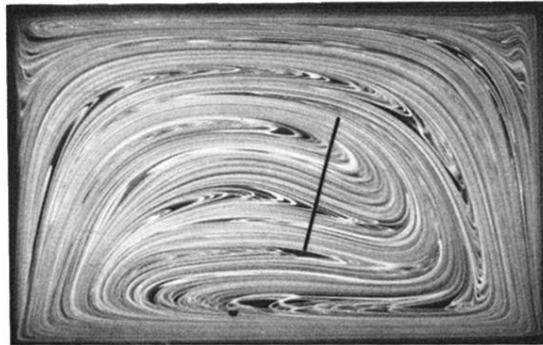
FIG. 1. Photograph showing typical structures produced by chaotic mixing in a cavity flow apparatus under creeping flow conditions (Ref. 1). Two fluids of about the same viscosity and negligible interfacial tension are mixed by moving the top and bottom walls of the cavity in a time-periodic fashion. A lamellar structure is generated, composed of thousands of striations of distributed thicknesses. The line represents a cut across the striations such as the one represented at the bottom of Fig. 2.
