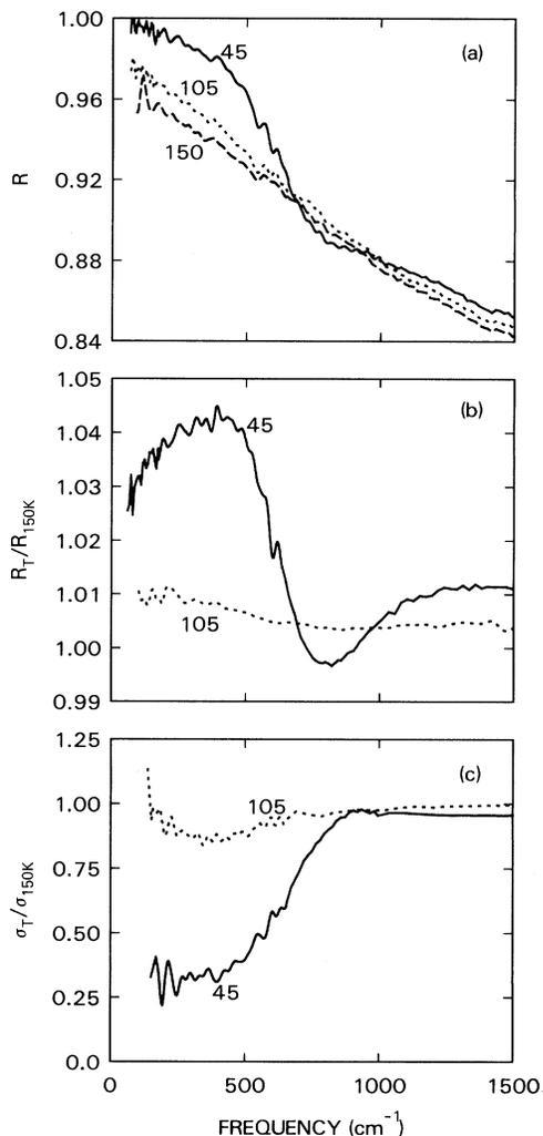
FIG. 1. (a) The  $a$ - $b$ -plane reflectivity of a  $\text{YBa}_2\text{Cu}_3\text{O}_7$  crystal at  $T=45$ , 105, and 150 K. (b) The  $a$ - $b$ -plane reflectivity at 45 and at 105 K, divided by that at 150 K. (c) The real part of the  $a$ - $b$ -plane conductivity at 45 and at 105 K divided by that at 150 K.
