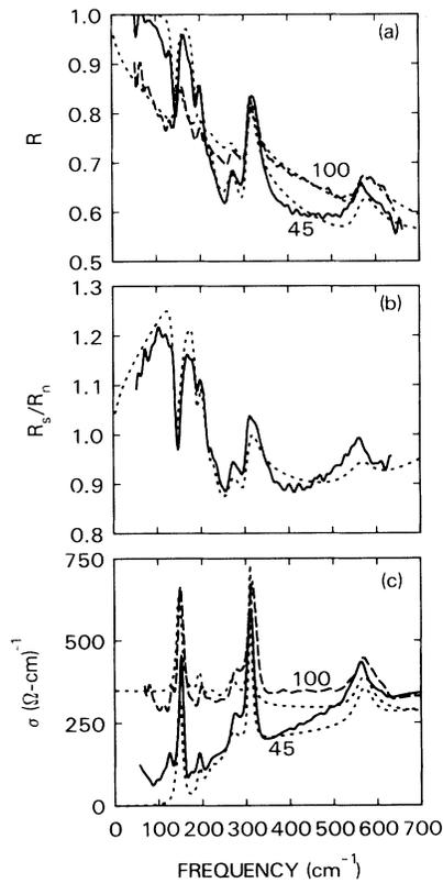
FIG. 3. (a) The reflectivity in the superconducting ( $T=45$  K) and normal ( $T=100$  K) states for the incident electric field along the  $c$ -axis direction. (b) The  $c$ -axis reflectivity in the superconducting state divided by that in the normal state. (c) The real part of the conductivity in the superconducting ( $T=45$  K) and normal ( $T=100$  K) states. The dotted lines are calculated fits to the data including both phonon and electronic contributions to  $\sigma(\omega)$ .
