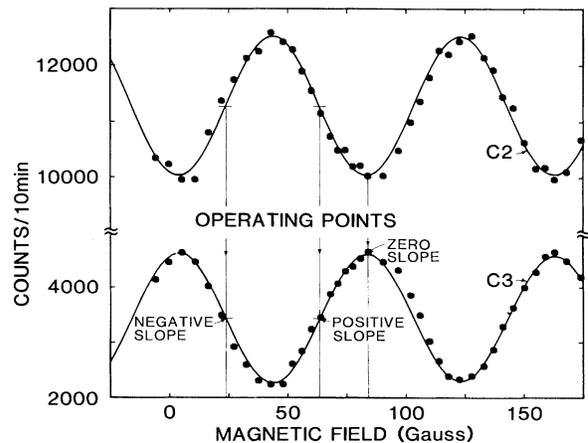
FIG. 3. Magnetic scan taken at an interferometer tilt angle of  $-1.10^\circ$ . The bias-magnetic-field operating points of negative, positive, and zero slopes of the  $C_3$  interferogram are indicated. The fact that  $\Delta\Phi_M = 0$  does not occur precisely at  $B = 0$  is due to fringing fields from the magnet.
