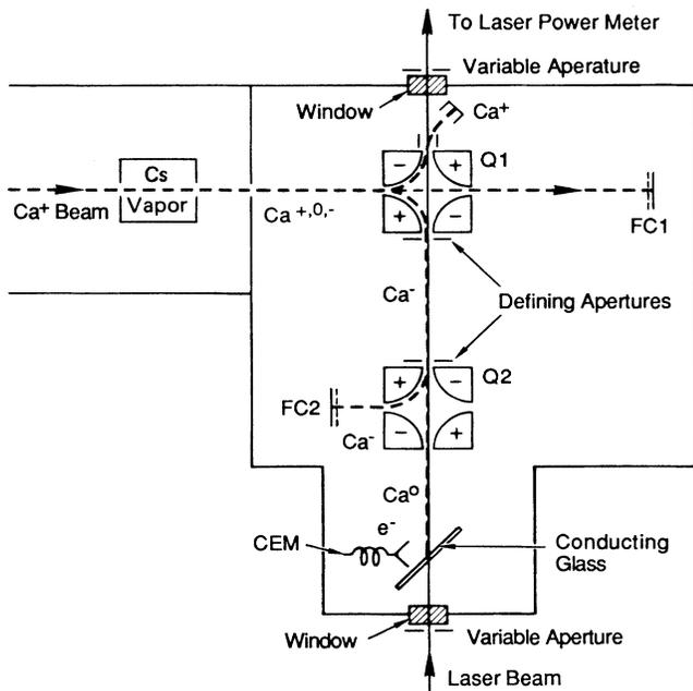
FIG. 2. Schematic diagram of the experimental setup.
