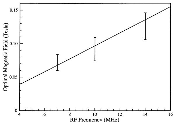
FIG. 4. Optimal magnetic field for maximum optical gain as a function of rf frequency.
