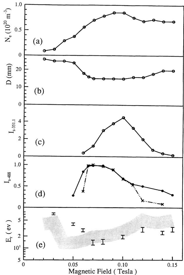
FIG. 3. (a) Electron density, (b) full width at half maximum of electron density, (c) spontaneous emission of ArIII 351-nm line, (d) small-signal optical gain, ×, and spontaneous emission, ●, of ArII 488-nm line, and (e) equivalent energy. All as a function of magnetic field, for rf power of 3.5 kW.
