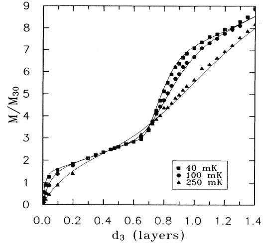
FIG. 3. Magnetization vs  $d_3$  at 40, 100, and 250 mK. Also shown is a fit by a two-level model having energy gap  $e_{12} \approx 1.8$  K near the step at  $d_3 = 0.74$  layer and a distribution in  $e_{12}$  of  $\sigma \approx 0.10$  K. We note that  $dM/dT \approx 0$  at  $d_3 = 0.71$ .
