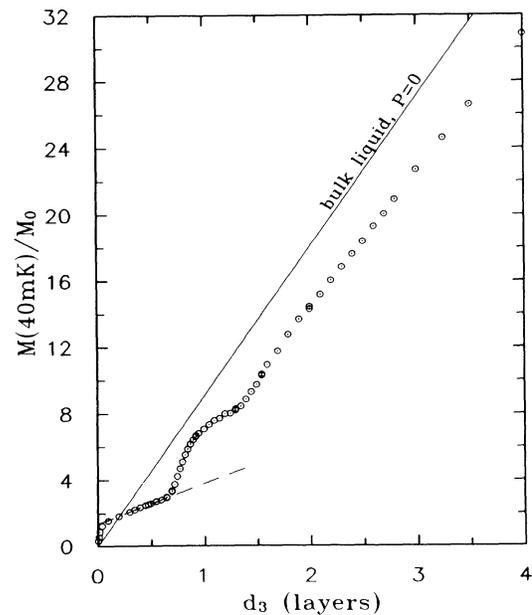
FIG. 2. Magnetization at  $T=40$  mK vs  $d_3$ , showing steps in magnetization at  $d_3 \approx 0.8$  and  $1.5$  layers, and an increase in magnetization with the same slope as for bulk liquid above  $d_3=2$  layers. The dashed line extrapolates low-coverage data to obtain the hydrodynamic mass  $m_h = 1.38m_3$ .
