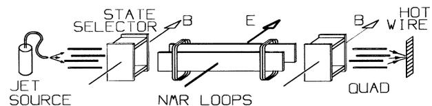
FIG. 1. Schematic view of the apparatus.
