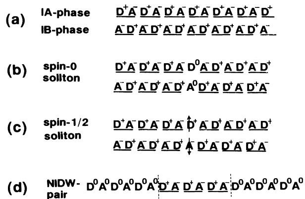
FIG. 1. Schematic structures of donor ( D ) and acceptor ( A ) stack: (a) dimerized stacks, (b) spin-0 solitons, (c) spin- \frac{1}{2} solitons, and (d) a pair of neutral-ionic domain walls (NIDW's).
