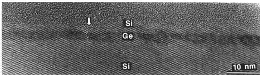
FIG. 2. Cross-sectional view of the sample presented in Fig. 1 (c). The arrow shows one defect.
