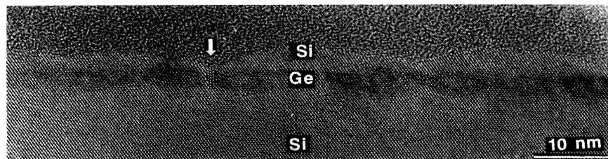
FIG. 2. Cross-sectional view of the sample presented in Fig. 1(c). The arrow shows one defect.
