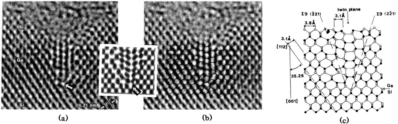
FIG. 3. (a) Detail of one defect. (b) Same defect, with atomic position superimposed (black-atoms assumption). (c) Atomic model of the defect. Inset between (a) and (b): Simulated image. The arrows on (a) and in the inset show the same atomic position, so that comparison between simulation and image can easily be done.
