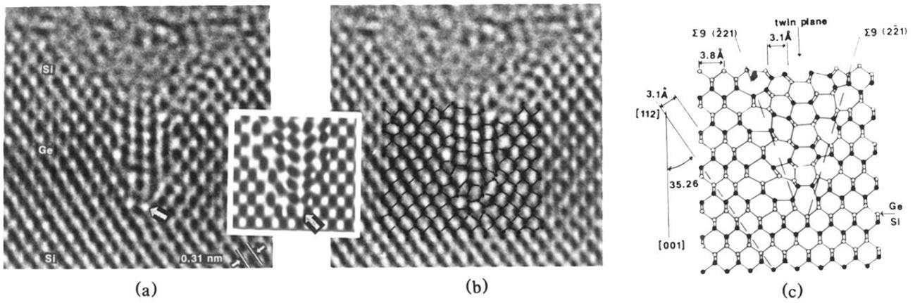
FIG. 3. (a) Detail of one defect. (b) Same defect, with atomic position superimposed (black-atoms assumption). (c) Atomic model of the defect. Inset between (a) and (b): Simulated image. The arrows on (a) and in the inset show the same atomic position, so that comparison between simulation and image can easily be done.
