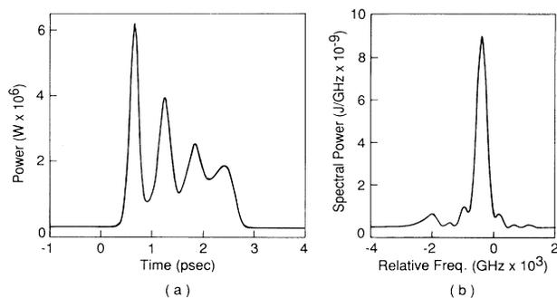
FIG. 2. Results of computer simulations using the MKIII parameters in Table I (Ref. 10). (a) Optical intensity profile as a function of time within a single micropulse. (b) Spectral power distribution as a function of difference in frequency from the laser fundamental.
