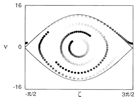
FIG. 1. Electron trajectories in phase space under highly saturated conditions. Time progresses from light gray to dark. Note the nearly circular orbits of some electrons [harmonic oscillation at  $\Omega = (c/L)|a|^{1/2}$ ]. This is the origin of the sidebands which result in the spiking behavior of free-electron lasers. (Courtesy W. Colson.)
