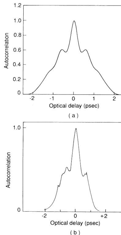
FIG. 3. (a) Autocorrelation function for the computed laser micropulse shown in Fig. 2. (b) Observed autocorrelation function during experiment, showing side lobes resulting from the spikes within the micropulse.
