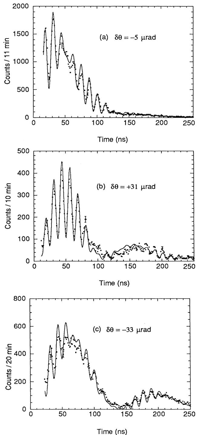
FIG. 1. Time distribution of resonantly scattered x rays from YIG (002) in symmetric Bragg geometry, with the indicated deviation angles from the Bragg angle (corrected for refraction due to the electron density). Each solid curve gives the intensity of the Fourier transform of the dynamical theory calculation for the multilevel energy-dependent reflectivity amplitude.
