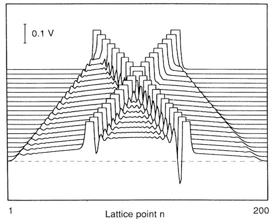
FIG. 5. The time evolution of an initial state given by an ideal two-soliton solution with  $R=20 \Omega$ ,  $G=0$ .
