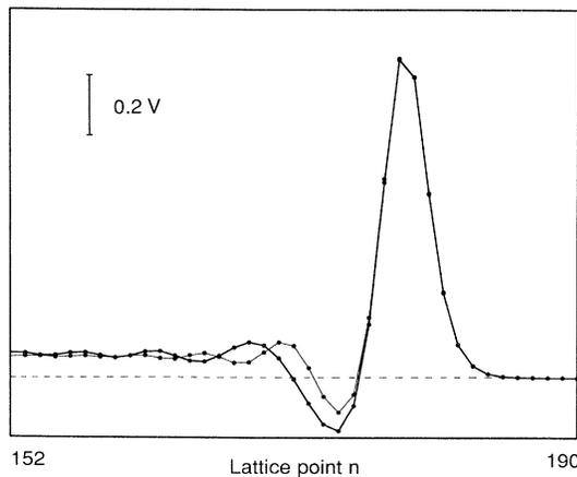
FIG. 4. Two one-soliton solutions with different initial amplitudes  $A=4.0 \text{ V}$  (thin line) and  $A=8.0 \text{ V}$  (thick line) recorded at a moment when they have the same amplitude. The taller soliton had traveled 3348 ns and the smaller 2374 ns.
