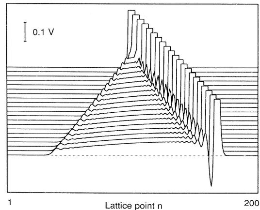
FIG. 2. The time evolution of an initial state given by an ideal one-soliton solution with  $R = 20 \Omega$ ,  $G = 0$ . The initial state is at the top. For clarity we have cut away the tops of the curves.
