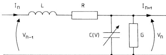
FIG. 1. A section of the nonlinear transmission line with resistance  $R$  and conductance  $G$ .
