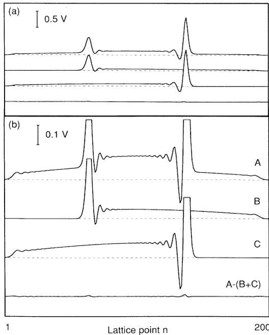
FIG. 7. (a) A two-soliton solution after the collision (*A*), two one-soliton solutions (*B* and *C*), and the result after the subtraction  $A - (B + C)$ ,  $R = 20 \Omega$ ,  $G = 0$ . (b) Same as in (a) but the vertical scale magnified by a factor of 6.
