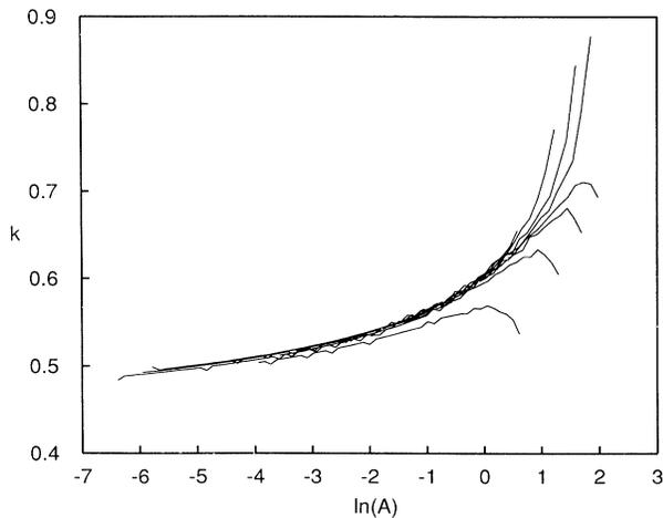
FIG. 3. The logarithmic derivative of the soliton amplitude  $k$  as a function of the logarithm of the amplitude  $A$  for different initial amplitudes and widths ( $R=20 \Omega$ ,  $G=0$ ). The initial states for the curves starting from the top were somewhat narrower than the ideal solitons (4).
