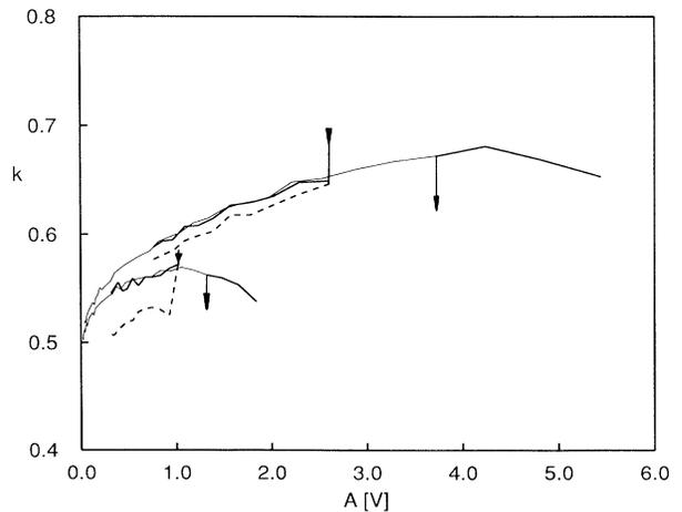
FIG. 9. The logarithmic derivative of the soliton amplitude  $k$  as a function of the amplitude  $A$  ( $R = 20 \Omega$ ,  $G = 0$ ) for the colliding solitons (thick line) with tail corrections (the behavior after collision without tail corrections is given by the dashed line). The decay of amplitude follows closely the behavior of the single soliton (thin line). The values of  $k$  during collision are not shown.
