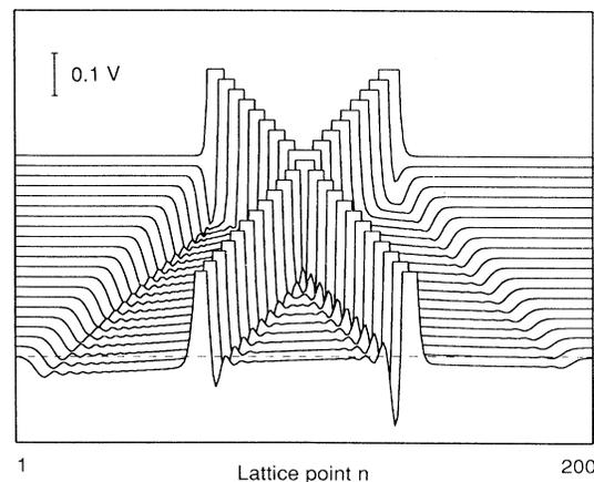
FIG. 6. The time evolution of an initial state given by an ideal two-soliton solution with  $R=0$ ,  $G=8.54 \times 10^5 \Omega^{-1}$ .
