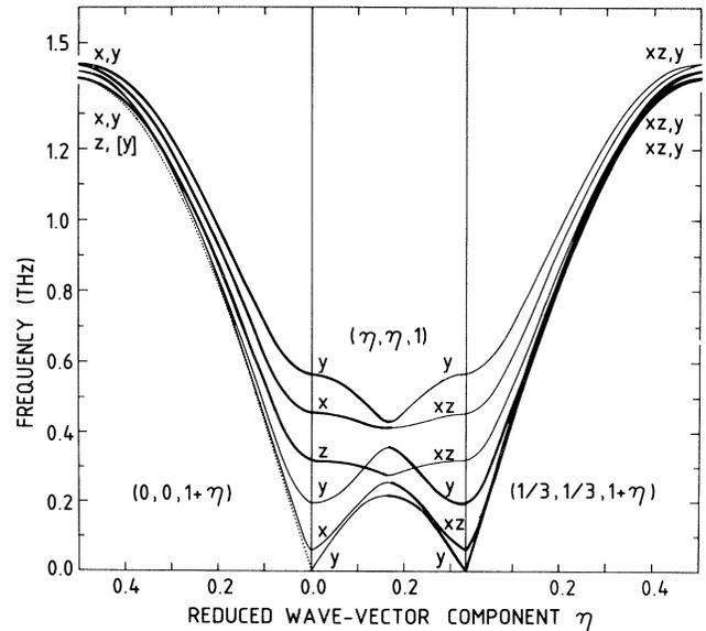
FIG. 1. The spectrum predicted by conventional spin-wave theory with  $D/6J' = -0.36$ , plotted vs  $(Q_a, Q_b, Q_c)$  from Ref. 5. Polarizations are indicated and line thickness corresponds to intensity.
