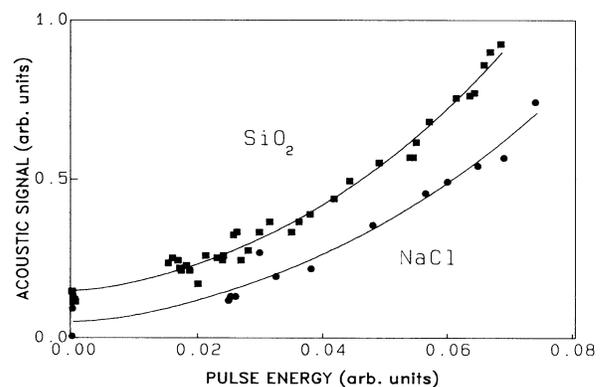
FIG. 1. Measured photoacoustic signal vs energy of 1064-nm pulses, obtained in NaCl (circles) and  $\text{SiO}_2$  (squares) under the constant pump condition. It shows clearly a nonlinear dependence on the energy of the heating pulse. The solid line for each measurement is the fit of Eq. (2) with the experimental data, showing a good agreement between theory and measurement.
