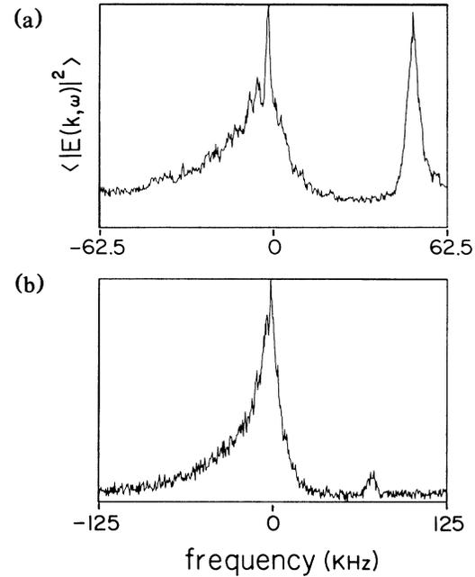
FIG. 2.  $\langle |E(\mathbf{k}, \omega)|^2 \rangle$  from two separate experimental runs. hf-heating pulses 10 ms long, at 150 ms IPP, and with  $\omega_0/2\pi = 7.3$  MHz were irradiated at an ERP of 60 MW. The radar pulse was delayed by (a) 0.5 ms and (b) 4 ms after the onset of the heater pulse, respectively. The frequencies are measured relative to  $\omega_0/2\pi$ .
