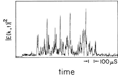
FIG. 4. (a) Real-time single-shot backscattered radar power signal,  $|\mathbf{E}(\mathbf{k}, t)|^2$ , from experiments. The signal was obtained by irradiating hf-heating pulses (10 ms, 150 ms, 7.3 MHz, 60 MW) and with the radar pulse delayed by 8 ms after the onset of the heater pulse.
