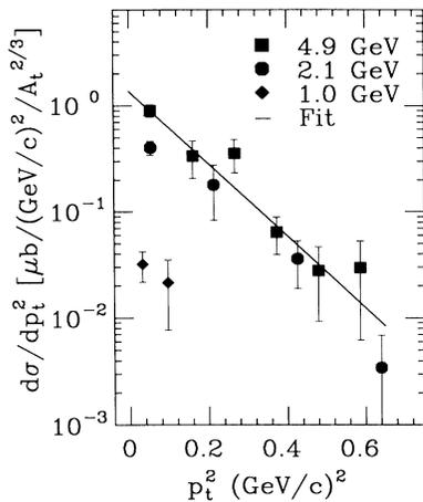
FIG. 2. The cross section per nucleon  $d\sigma/dp_t^2$  as a function of  $p_t^2$  for three beam energies. The solid line is a fit to the 4.9-GeV data [ $\exp(-7.8p_t^2)$ ].
