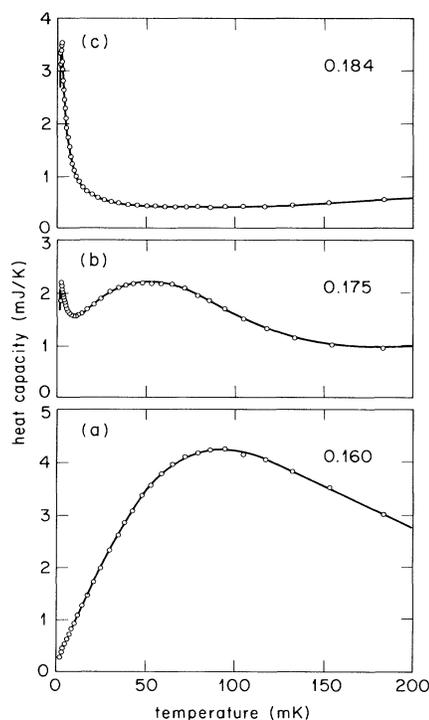
FIG. 1. Heat-capacity data at three coverages near third-layer promotion which show that the second  $^3\text{He}$  layer undergoes a first-order transition. The numbers give the coverages in atoms per square angstrom.
