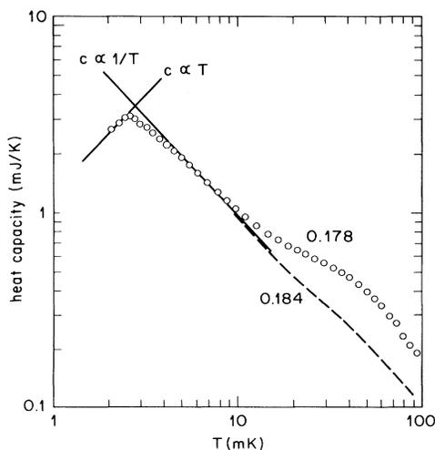
FIG. 3. Nuclear-spin contribution to the heat capacity of the second-layer registered phase. The numbers give the coverages in atoms per square angstrom.
