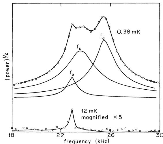
FIG. 1. The Fourier-transform power spectra of the data (open squares) and our fits (solid lines). We show a  $H_0 = 7$  G line broken into its three components along with a magnified liquid line that was recorded at 12 mK.
