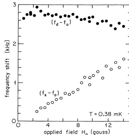
FIG. 2. Field dependence for the frequency shifts of the two modes relative to the Larmor frequency. The open circles record the shifted-mode frequency difference  $f_s - f_0$  which is linear in the applied field. The closed circles record the displaced-mode frequency difference  $f_d - f_0$  that shows an almost constant displacement of 2.7 kHz above the Larmor frequency.
