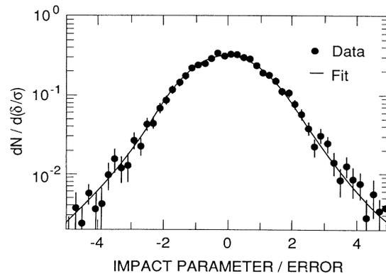
FIG. 1. Impact-parameter/error distribution for hadron tracks having small fractions of their transverse momenta in the plane perpendicular to the beams. The fitted curve represents the resolution function.
