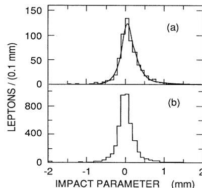
FIG. 2. Impact-parameter distributions for (a) leptons in the  $b$ -enhanced region and (b) hadrons in the same  $p$  and  $\bar{p}$  region. The curve represents the result of the fit described in the text for the measured lifetime.
