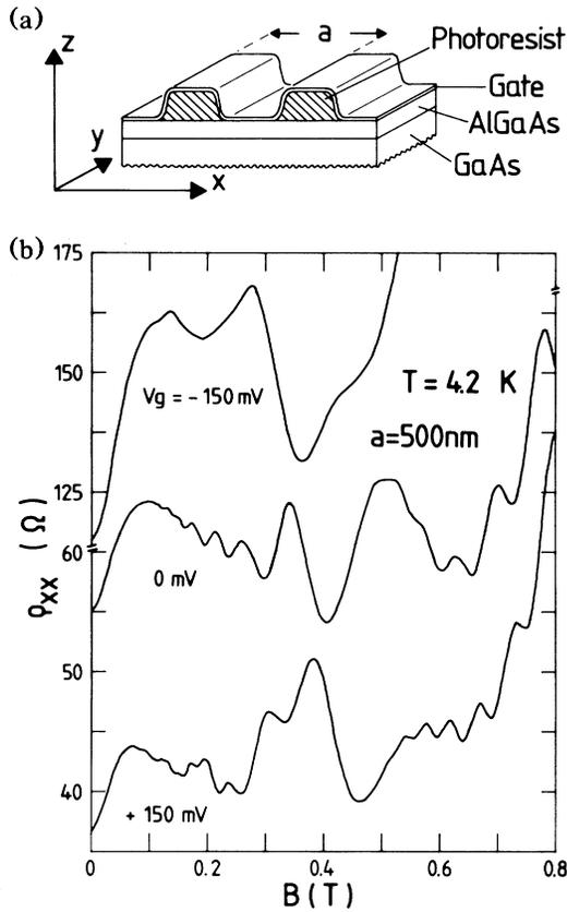
FIG. 1. (a) Schematic cross section of a heterojunction with a periodic gate structure. (b) Measured  $\rho_{xx}$  vs magnetic field  $B$  for three different gate voltages  $V_g$ .
