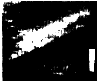
FIG. 3. This image demonstrates the feasibility of direct imaging of biological specimens with the PRM, and also demonstrates materials contrast. A single strand of hair is placed on a silver-foil conducting substrate (dark background). This substrate was chosen for its low e^+ reemission [ P(E)\approx 0.3\% ], highlighting the high specimen reemission [ P(E)\sim 2\% ]. The magnification is M=15\times and R=15\ \mu\text{m} . The image required 20 h of signal averaging to accumulate. The white bar represents 100\ \mu\text{m} . Sample charging may have contributed to degraded image quality and resolution.
