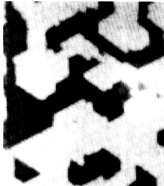
FIG. 1. 470 \times 400\text{-}\text{\AA}^2 tunneling image of 1-ML Ga-covered Si(111), showing the overlayer superlattice of 24\text{-}\text{\AA} periodicity, with (3.2 \pm 0.2)\text{-}\text{\AA} step heights. The tip bias and tunneling current are -3.32 \text{ V} and 800 \text{ pA} , respectively.
