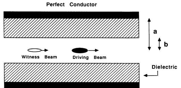
FIG. 1. Sketch of the dielectric cavity.
