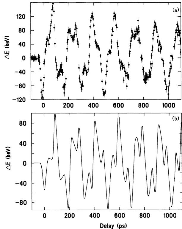
FIG. 3. Steatite scan: (a) measured and (b) calculated wake potential.
