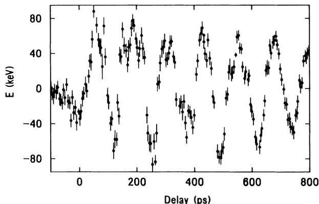
FIG. 4. Nylon scan: Wake potential measured as a function of witness-bunch delay.
