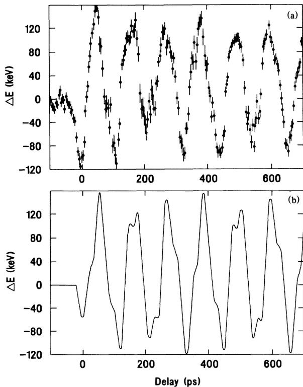
FIG. 2. Polystyrene scan: (a) measured and (b) calculated wake potential.
