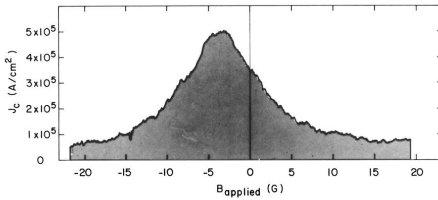
FIG. 5. Critical-current density vs applied magnetic field (perpendicular to the film) at 5 K for a 5° grain boundary.
