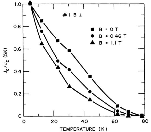
FIG. 3. Normalized critical-current density vs temperature for sample No. 1 (compare with Fig. 2) in magnetic fields perpendicular to the film. This particular sample showed a pronounced tail in the  $J_c(T)$  characteristic for  $T > 65$  K.
