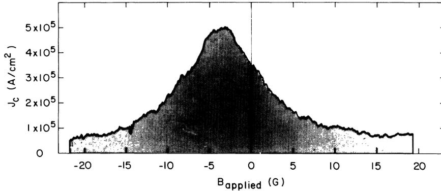
FIG. 5. Critical-current density vs applied magnetic field (perpendicular to the film) at 5 K for a  $5^\circ$  grain boundary.
