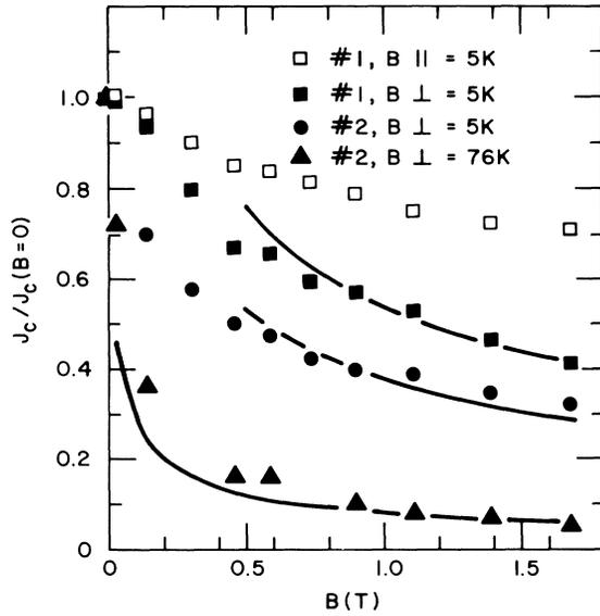
FIG. 2. Normalized basal-plane critical-current densities vs  $B$  for two samples. The magnetic fields are oriented to the film plane as indicated, but are always perpendicular to the transport current.  $J_c(0)$  equals  $1.3 \times 10^6$  and  $4 \times 10^6$  A/cm<sup>2</sup> for samples No. 1 and 2, respectively.
