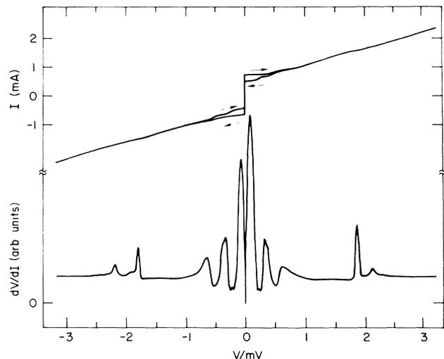
FIG. 4.  $I(V)$  and  $dV/dI(V)$  characteristic at 5 K for a 37° grain boundary.
