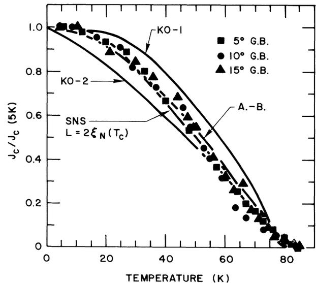
FIG. 6. Normalized critical-current density vs temperature for three grain boundaries. KO-1 and KO-2 are the dependences predicted by Kulik and Omel'yanchuk for weak links in the dirty and in the clean limits, respectively. The curves labeled AB and SNS refer to the theories of Ambegaokar-Baratoff and Likharev, respectively.
