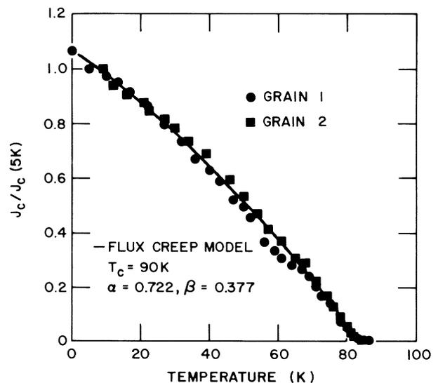
FIG. 1. Normalized critical-current densities vs temperature for two  $c$ -axis grains. The solid line is a fit by the flux creep model.  $J_c(0)$  equals roughly  $6 \times 10^6 \text{ A/cm}^2$  for both grains.
