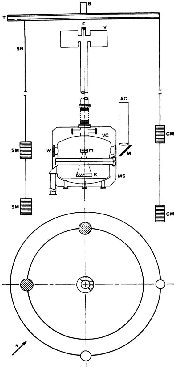
FIG. 1. Sketch of the apparatus, along with the plan view; B=bearing, T=truss, F=fiber holder, SR=suspension rods, V=ion pumps, SM=source masses, CM=counterweights, VC=vacuum chamber, W=optically flat windows, m= $\lambda/20$  mirror, M= $45^\circ$  mirror, AC=autocollimator, R=ring, and MS=magnetic shield.
