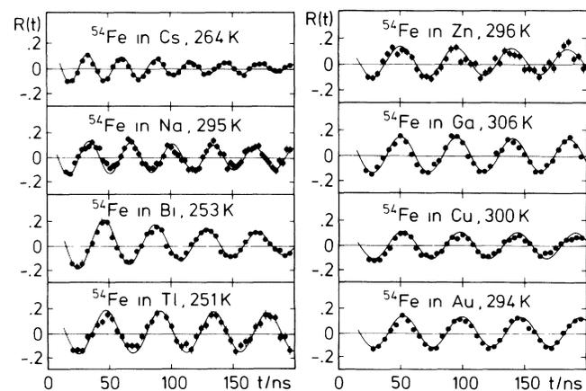
FIG. 1. Host dependence of the spin rotation of  $^{54}\text{Fe}$  in several *sp* metals and in Cu and Au observed in an external field of 2 T.
