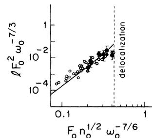
FIG. 2. Scaled values of localization length  $l_e$ , following Refs. 5 and 15. The open circles are numerical results based on quantum mechanics, the filled circles are the experimental data of Table I, and the solid line follows from a model localization theory. The vertical dashed line is the theoretically predicted quantum delocalization border (Refs. 5 and 15).
