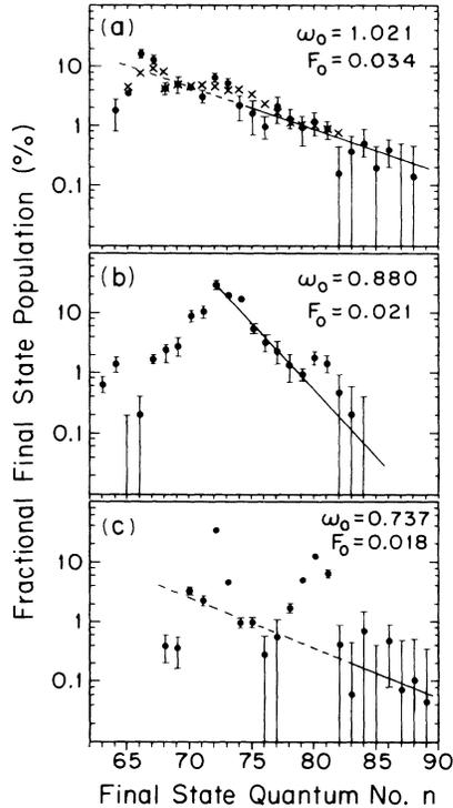
FIG. 1. Experimental final-bound-state quantum number distributions for three pairs of values of classical scaled microwave frequency  $\omega_0 = n_0^3 \delta \omega$  and peak microwave field strength  $F_0 = n_0^4 F$ . The error bars are an rms measure of overall data reproducibility. Values of experimental distribution length are obtained from the solid straight lines. For case (a), the crosses are numerical predictions assuming classical physics, from Ref. 11.
