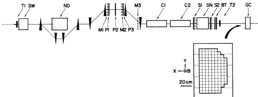
FIG. 1. Elevation view (not to scale) of the secondary beam line and the experimental arrangement, and front view of the electromagnetic calorimeter.
