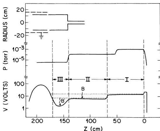
FIG. 1. A schematic diagram of the positron trap showing the electrodes surrounding the confinement region (region III) and the nitrogen-gas pressure and potential profiles along the direction of the axial magnetic field.
