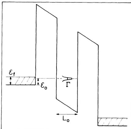
FIG. 1. Schematic band-edge diagram for a semiconductor double-barrier resonant-tunneling structure. The center of the resonant level is an energy  $\epsilon_0$  above the band edge in the injecting lead, and the full width of the resonant level is given by  $\Gamma$ . The width of the quantum well is  $L_0$ .
