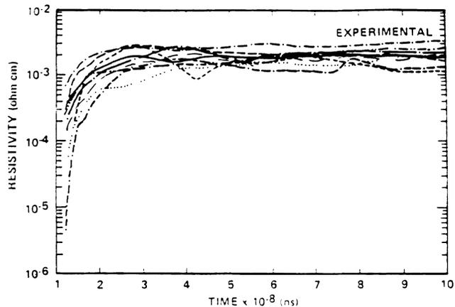
FIG. 2. Resistivity vs time for nine shots.
