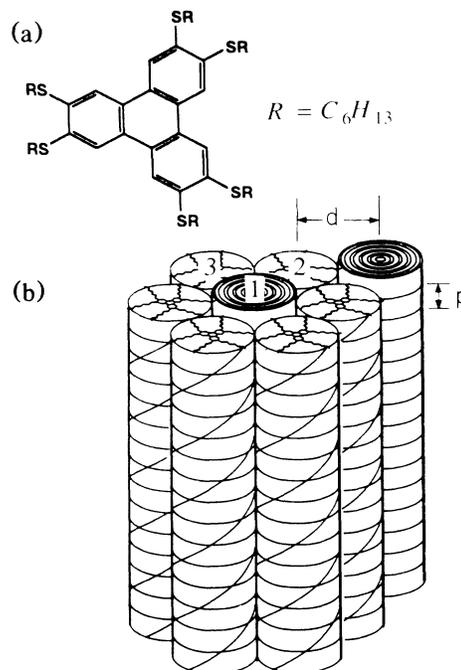
FIG. 1. (a) Hexa-hexylthiotriphenylene (HHTT). (b) Proposed structure of three-column superlattice (not to scale). Column 1 has random average helical phase, and is displaced by  $p/2$  from columns 2 and 3, which have correlated phases.
