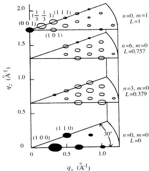
FIG. 2. Perspective schematic of diffraction pattern. Circle sizes are proportional to  $\log(I)$ ; we measured 14700 and 1.7 counts/s in the (100) and (300) peaks, respectively. Open circles indicate peaks observed in the  $D_{ho}$  phase only; filled circles, those found in both  $D_{ho}$  and  $D_{hd}$  phases.
