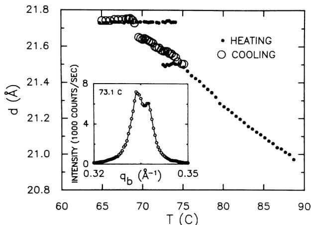
FIG. 3. Intercolumnar distance  $d$  vs temperature. Filled circles indicate measurements made on warming; open circles, measurements on cooling. Inset: a typical coexistence profile of the (100) peak, at 73.1 C.
