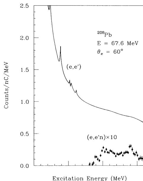
FIG. 1. Inclusive ( $e,e'$ ) and coincident ( $e,e'n$ ) spectra from  $^{208}\text{Pb}$ . The coincidence condition removes the radiative tail, revealing the nuclear response.
