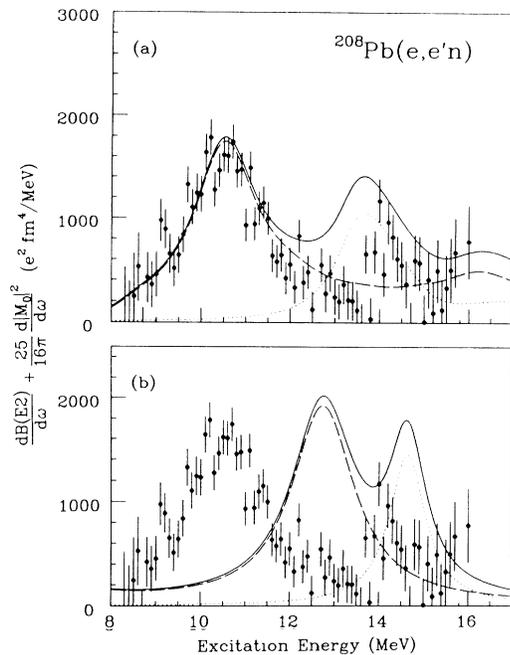
FIG. 2. The sum of the  $E0$  and  $E2$  nuclear responses, as inferred from the  $^{208}\text{Pb}(e,e'n)$  measurements, compared to (a) the RPA calculation of Wambach and Co' (Ref. 25) and (b) the TDHF-RPA calculation of Dechargé and Gogny (Ref. 27). The solid curve gives the total  $E0/E2$  response. The dotted and the dashed curves give the monopole and quadrupole responses, respectively.
