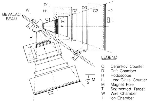
FIG. 1. The DLS experimental setup.
