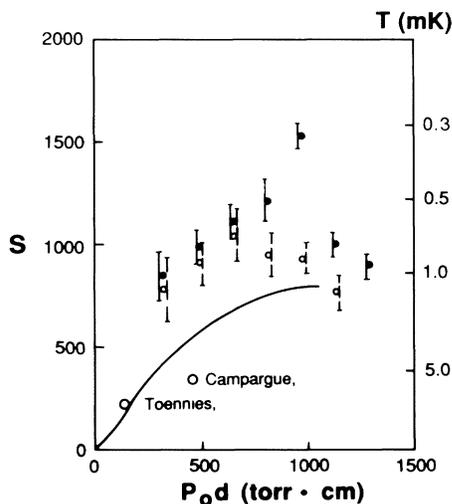
FIG. 2. Speed ratio  $S$  and parallel temperature  $T$  as functions of the  $P_0d$  product. The filled and open circles correspond to measurements with nozzle-skimmer distances of 1.12 and 0.44 m, respectively. For comparison, the largest  $S$  values reported by Campargue (Ref. 19) and Toennies and co-workers (Ref. 20) are also given, along with the theoretical predictions (solid line) of Toennies and Winkelmann (Ref. 20).
