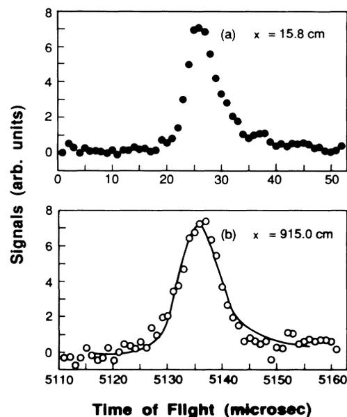
FIG. 1. TOF distributions measured at two distances  $x$  from the chopper. Both signals are actually negative with respect to those for the unchopped beam, as explained in the text, but have been inverted in these figures so as to show peaks in the conventional way. The solid line in part (b) is the best fit from convolving a Gaussian speed distribution with the signal shown in part (a).
