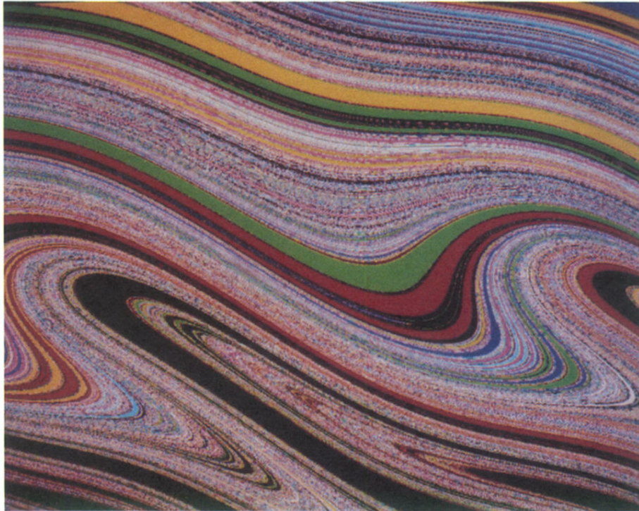
FIG. 5. Supercomputer simulations for a 750 \times 750 grid in color. Vertical axis: initial condition in the pendulum velocity. Horizontal axis: initial condition in the pendulum angle. See text for discussion of colors.
