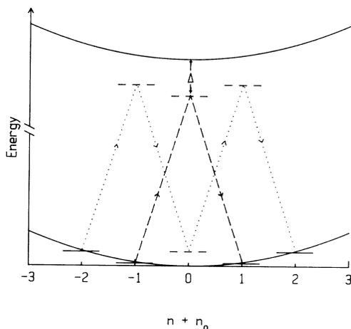
FIG. 3. Energy levels of the momentum eigenstates determined by their respective kinetic energies;  $E_n = (n+n_0)^2 \times (25 \text{ kHz})$ . First-order Bragg scattering (dashed lines) can be viewed as a two-photon transition from the undiffracted ( $n+n_0 = -1$ ) to the diffracted ( $n+n_0 = 1$ ) state. Second-order Bragg scattering (dotted lines) can be viewed as two two-photon transitions from the undiffracted ( $n+n_0 = -2$ ) to the diffracted ( $n+n_0 = 2$ ) state.
