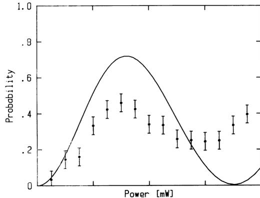
FIG. 4. Plot of probability to be in the diffracted ( $n+n_0=1$ ) state as a function of laser power,  $\Omega_0^2\tau$ , for first-order Bragg scattering ( $n_0=-1$ ):  $\Delta=800$  MHz and  $\tau=5$   $\mu$ s ( $\Delta w=2.5$  mm) for these plots. Also shown are experimental data of population in the diffracted state for various laser powers.
