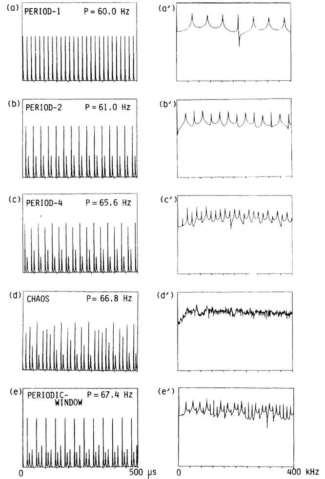
FIG. 2. (a)–(e) PQS-pulse trains and (a')–(e') their power spectra as functions of the pumping rate  $P$  obtained from numerical calculations based on the three-level:two level rate-equation model. The power spectra are plotted in logarithmic units.
