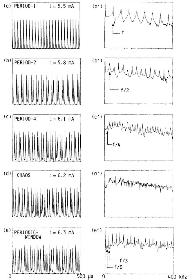
FIG. 1. (a)–(e) PQS-pulse trains and (a')–(e') their power spectra observed as functions of the discharge current  $i$ . The power spectra are plotted in logarithmic units. The chaotic pulsation [(d)] appears following the period-doubling bifurcation [(a)–(c)]. A periodic window [(e)] appears at 6.3 mA.
