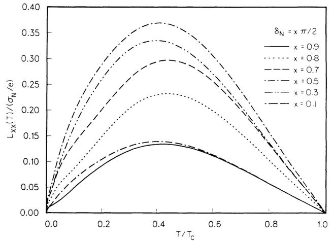
FIG. 1. Thermoelectric coefficient  $I_{xx}$  as a function of temperature for the  $d$ -wave state described in the text.
