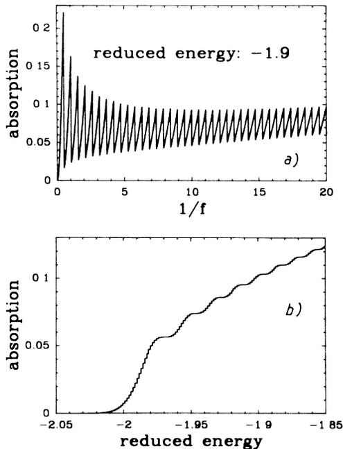
FIG. 2. (a)  $f^{-1}$  oscillations of the absorption at a fixed reduced photon energy close to the SL band gap, calculated for a 201-period SL. (b) Convergence of the SL absorption toward the Franz-Keldysh oscillations, calculated for a 4001-period SL and a very small reduced electric field  $f=1.5 \times 10^{-3}$ .
