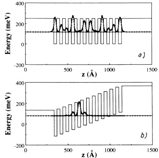
FIG. 3. Sketch of the heterostructure considered in the numerical approach, (a) at zero electric field and (b) in a discretized potential simulating an electric field of 30 kV/cm. Also shown is the square of the modulus of the eigenfunction corresponding to a state near the center of the miniband. Calculations are made with use of the band parameters of the GaAs-Al<sub>0.3</sub>Ga<sub>0.7</sub>As system, and well and barrier thicknesses of 35 Å.
