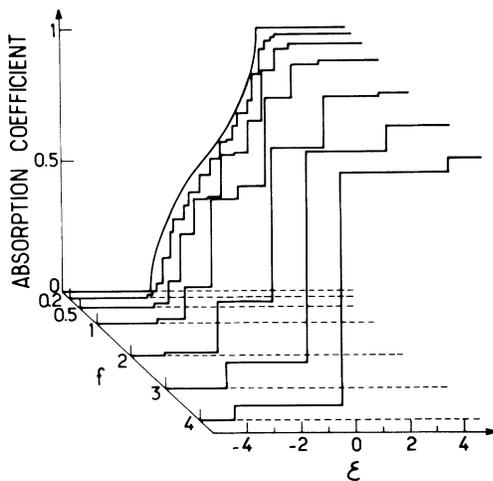
FIG. 1. Absorption of a 41-period superlattice, normalized to  $(2N+1)\alpha_0$ , vs the reduced photon energy  $\epsilon = [\hbar\omega - (E_g + E_1 + H_1)]/(\lambda_c + \lambda_v)$ , for increasing values of the reduced electric field  $f = eFd/(\lambda_c + \lambda_v)$ .
