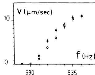
FIG. 5. Propagation velocity  $v$  at threshold as a function of the frequency  $f$ , showing the transition at  $f_1 = 530$  Hz from the stationary to the time-dependent state.
