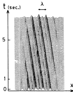
FIG. 3. Time dependence of an optical density profile along  $\mathbf{x}$  showing motion to the left. The period between two successive profiles is 0.12 sec. The wavelength is  $\lambda = 2d = 60 \mu\text{m}$  and the domain contains five wavelengths. Here  $\epsilon = 0.3$ .
