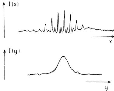
FIG. 2. Optical density profiles fitted to a soliton profile  $\text{sech}^2$  (dotted lines):  $I(x)$  is along the direction normal to the rolls ( $\mathbf{x}$ ),  $I(y)$  along a roll ( $\mathbf{y}$ ).
