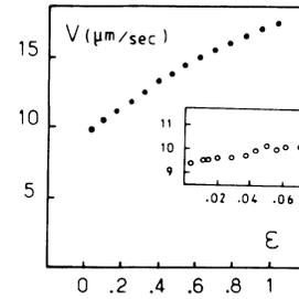
FIG. 4. Velocity of propagation vs reduced voltage. Inset: Velocity is finite close to threshold.
