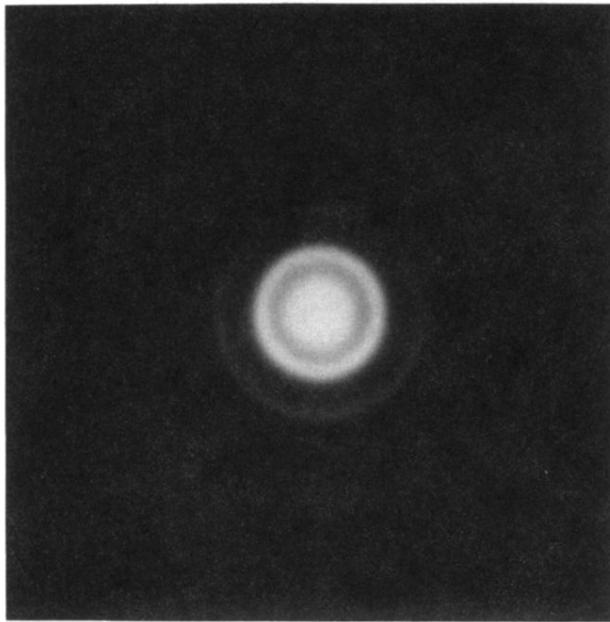
FIG. 2. Selected-area electron diffraction pattern taken from the central region of the indentation in Fig. 1. The concentric rings are characteristic of an amorphous structure.
