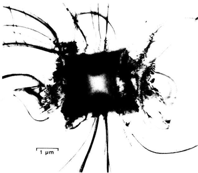
FIG. 1. Bright-field transmission electron micrograph of an indented region in a single crystal of Si. Note the lack of penetration of the bend contours into the grey, central region of the indentation.
