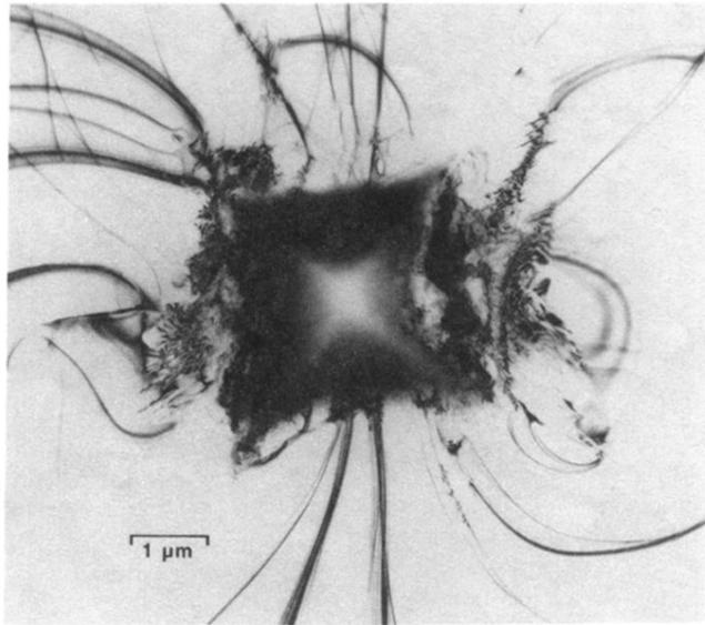
FIG. 1. Bright-field transmission electron micrograph of an indented region in a single crystal of Si. Note the lack of penetration of the bend contours into the grey, central region of the indentation.
