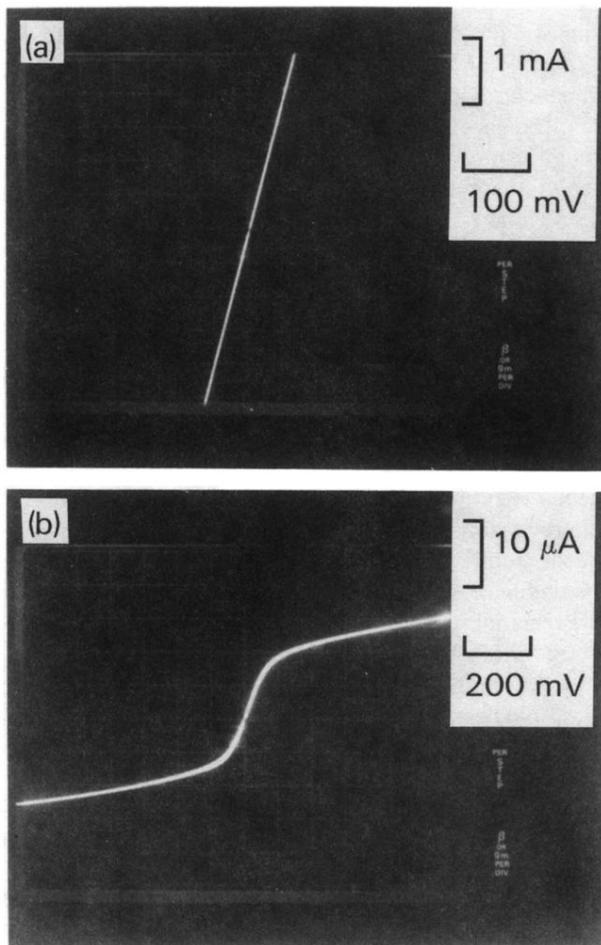
FIG. 3. Electrical conductivity behavior for Si between the electrodes described in the text (a) during indentation contact (under load) and (b) before (and after) indentation contact. The change in scale indicates an increase in conduction of 2 orders of magnitude between (b) and (a).
