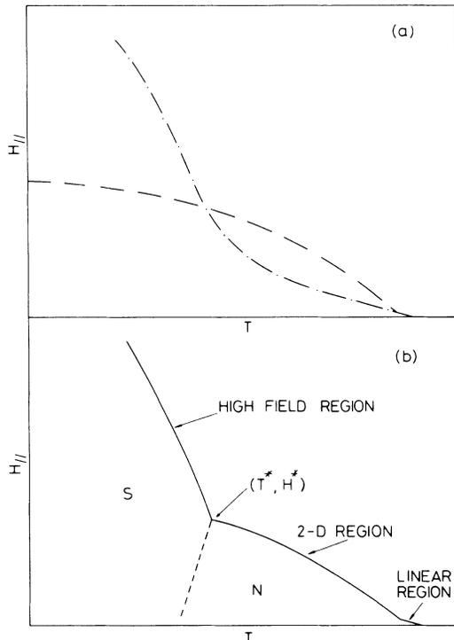
FIG. 1.  $H_{c2||}$  vs  $T$  after Ref. 6. In (a) the dashed line represents  $H_{c2||}(T)$  when  $\Delta(r)$  nucleates in the  $n$  (clean) layers whereas the dash-dotted line is the result of  $\Delta(r)$  nucleating in the  $s$  (dirty) layers. The solid line in (b) is the theoretically predicted result and the dashed line is the expected separation between the two regions.
