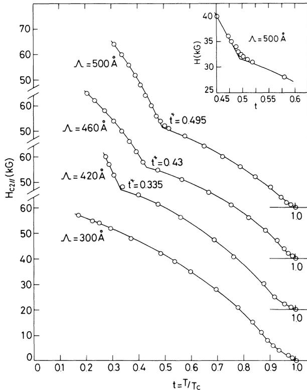
FIG. 2. Resistivity measured  $H_{c2||}$  vs  $t$  ( $=T/T_c$ ). The  $y$  axes are displaced for clarity and the solid lines are guides to the eye. Inset: Blowup of the region around  $t^*$  for the 500-Å sample.
